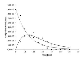
**Fig. 6** Experimental ethanol photodegradation tests performed using the A-HR catalyst. Empty points represent acetaldehyde. Dotted lines are the simulated trends obtained using the regressed kinetic constant.
