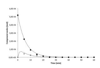
Fig. 4 Experimental ethanol photodegradation tests performed using the P25 catalyst. Empty points represent acetaldehyde. Dotted lines are the simulated trends obtained using the regressed kinetic constant.
