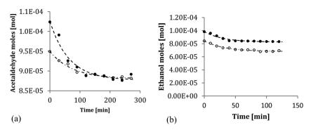
Fig. 3 Adsorption runs of (a) acetaldehyde and (b) ethanol on P25 (○) and 1077 (●). Dotted lines are the calculated curves using the regressed adsorption constants.
