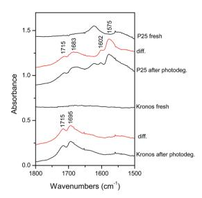
Fig. 7 Absorbance FTIR spectra relative to fresh and used P25 (top spectra) and 1077 (bottom)  $TiO_2$  samples in the ethanol degradation reaction. The differences between the spectra of the samples before and after ethanol degradation are reported in red.
