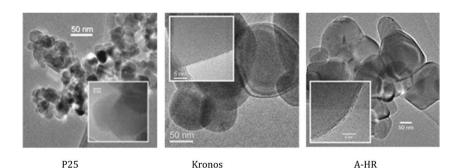
Fig. 1 TEM images of the various  $TiO_2$  samples.
