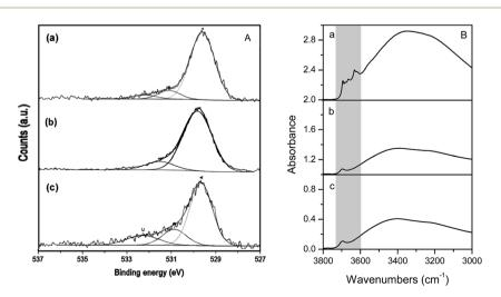
Fig. 2 O<sub>1s</sub> XPS spectra (A) and FTIR spectra (B) recorded at RT in air for (a) P25, (b) A-HR, (c) 1077.
